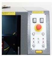
Switch on the laser controller PC by pressing the power button on its front panel. A Blue indicator light will appear. The controller will start up quickly and display the familiar desk top display.
