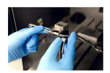
Clean off the excess GMS fluid which has not been bonded to the instrument, by wiping it off with a detergent wipe.
