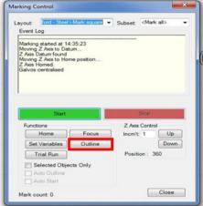
The green Start and red Stop buttons on the making control display perform the same functions as the green and red illuminated buttons on the Laser front panel.
